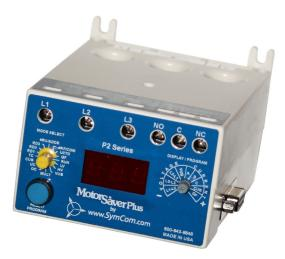
SymCom's Model 777-575-LR-HRG-P2 is a fully programmable electronic overload relay that is designed for resistively grounded systems. The 777-575-LR-HRG-P2 is recommended for monitoring and protecting any 3-phase 500-600VAC motor, used in a high resistance grounded (HRG) system, drawing 91-800 full load amps (external CTs are required). The units provide unsurpassed protection from faulty voltage and current conditions.
